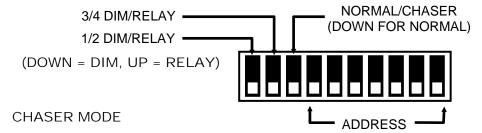
When operating in the chaser mode the AS-40L becomes independent of the control console and other dimmers. The green LED indicator is OUT when in the chaser mode. Chaser mode is turned on and off by one of the DIP switches on the end of the unit. A diagram on the unit cover shows the switch settings for controlling chaser operation.
