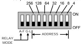
Any switch in the up position ADDS the associated value to the starting channel number. All switches down = starting channel number 1.
