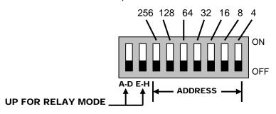
Any switch in the up position ADDS the associated value to the starting channel number. All switches down = starting channel number 1.
