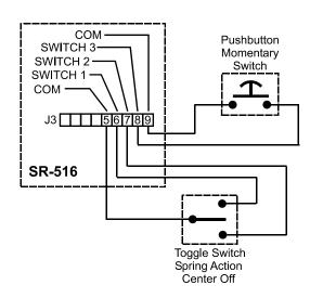
The example uses a Lightronics APP01 switch station and a momentary pushbutton switch. If the SR-516 simple switch functions are set to factory default operation then the switches will operate as follows.
