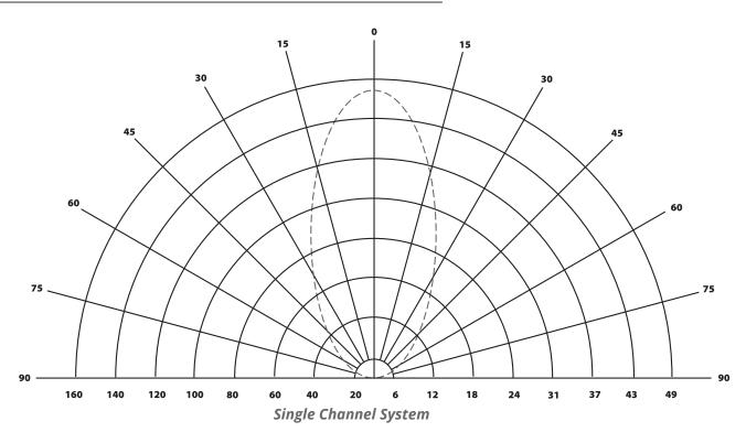
It is a good idea to provide over-lapping coverage (like in a sprinkling system) of the signal whenever possible to ensure that the signal does not have drop outs. In addition, you should provide special radiator coverage for shaded areas such as under a balcony or in the front of a room where the front mounted radiators do not provide enough coverage. The following diagrams illustrate these concepts.
