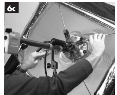
5 First slightly loosen Tilt Lock on SoftCore (arrow). Then loosen extension collar lock on Half Pole. Extend Half Pole carefully to get a working balance of the SoftCore, lamphead/lamps, and Pole counter-balance on stand. Tighten Tilt Lock on SoftCore, and lock Collar Knob on Half Pole. Note: be prepared to adjust balance after adding the softbox.
