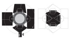
**Use the rotating barndoors** to trim unwanted output spill, (for example: to reduce risk of shadow in your shot caused by use of overhead boom microphones). Flexi-shafts & Tota-flags can also be attached for increased light control options.
