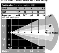
Beam angles-points at which intensity drops to 50% of maximum
