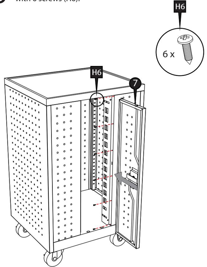
**7** Attach the left and right front doors (8 & 9) to the assembly with 12 screws (H6).
