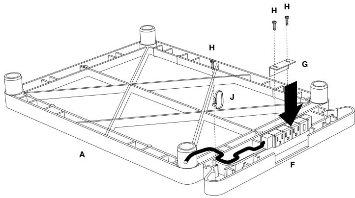
Attach electric outlet **F** to top shelf **A**, secure with L bracket **G** and cable lock **J**. Loop outlet cable **F** through cable lock **J** and the inserts on shelf **A**. Screw L bracket **G** and cable lock **J** onto top shelf **A** with screw **H** and a philips screwdriver.
