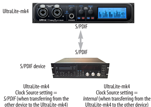
Figure 4-2: The setup for synchronizing a S/PDIF device with the UltraLite-mk4. Sync is achieved via the digital I/O connection itself. In this case, you have to choose S/PDIF as the UltraLite-mk4’s clock source when recording from the other device.
