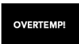
When the amplifier has cooled down to a safe operating temperature, the thermal switch resets itself, and the DLM loudspeaker resumes normal operation.
