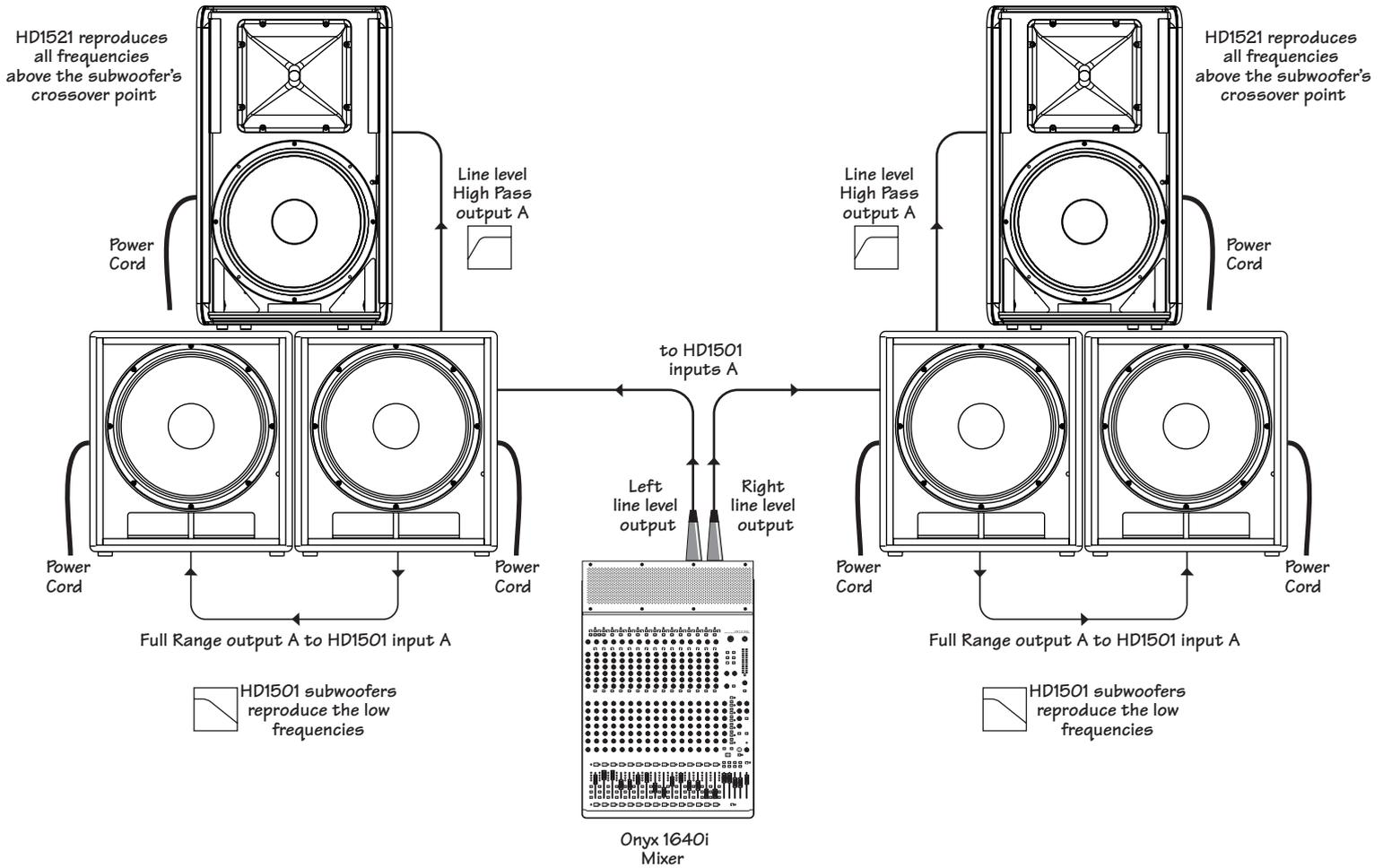
*This diagram shows the left and right line level outputs of a Mackie Onyx 1640i mixer feeding input A of two Mackie HD1501 subwoofers. The Full Range output A of each subwoofer then feeds input A of another pair of Mackie HD1501 subwoofers. The High Pass output A of these subwoofers also feed the input of each Mackie HD1521 loudspeaker. Be sure to disengage the Polarity Invert switch on the HD1501 subwoofers to optimize performance. See page 10 for more information.*
