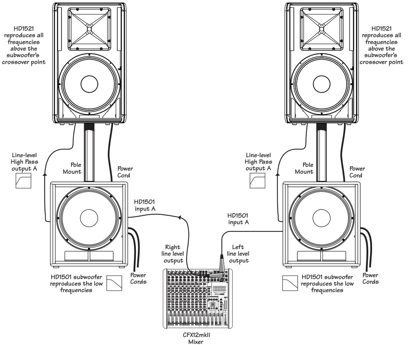
This diagram shows the left and right line level outputs of a Mackie CFX12mkII mixer feeding input A of two Mackie HD1501 subwoofers. The High Pass output A of each subwoofer then feeds the input of each Mackie HD1521 powered loudspeaker. Experiment with the HD1501's polarity switch to achieve optimum performance. Placement of the subwoofer relative to the full-range loudspeakers will also affect performance. See page 10 for more information.
