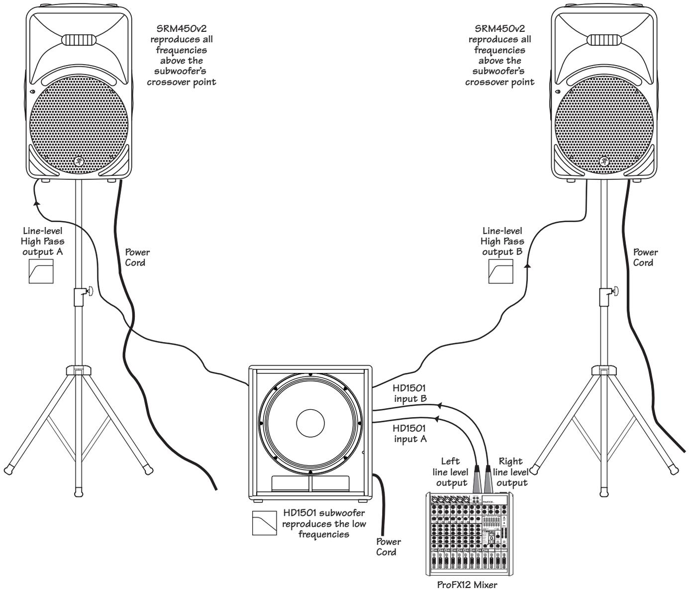
*This diagram shows the left line level output of a Mackie ProFX12 mixer feeding inputs A and B of one Mackie HD1501 subwoofer. Two SRM450v2 powered loudspeaker inputs are fed from the A and B High Pass outputs from the subwoofer. Experiment with the HD1501's polarity switch to achieve optimum performance. Placement of the subwoofer relative to the full-range loudspeakers will also affect performance. See page 10 for more information.*
