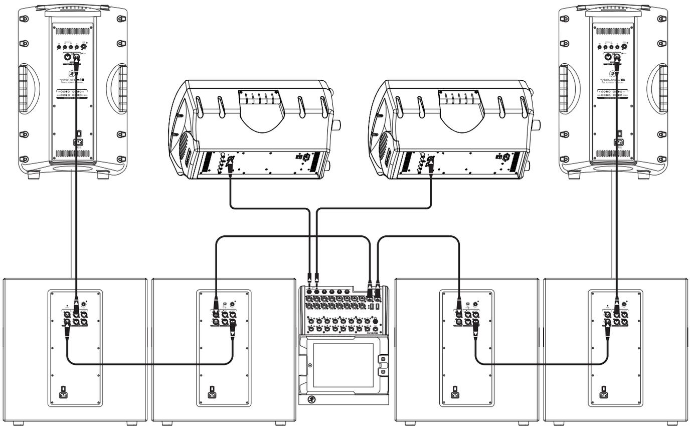
Here's how to set up a large club system. In this example, the L/R outputs of a DL1608 mixer are connected directly to the channel A inputs of two Thump18S subwoofers. The channel A full range outputs of these two Thump18S subwoofers are connected directly to the channel A inputs of another set of Thump18S subwoofers. Talk about beefy low end...and we've only connected the subs!
