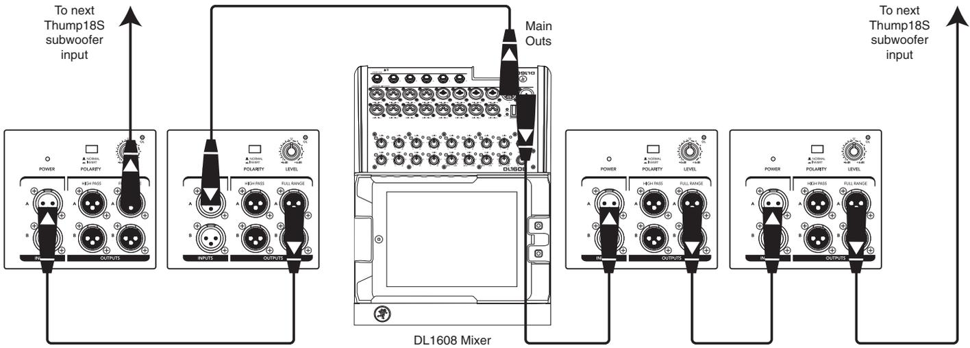
*Thump18S subwoofers may be daisy-chained via the male XLR connector labeled "FULL RANGE". Simply plug the signal source (i.e., mixer output) into the input jack(s), and patch that subwoofer's full range jack to the next subwoofers's input jack, and so on, daisy-chaining multiple Thump18S subwoofers. See above for a visual representation of daisy-chaining.*
