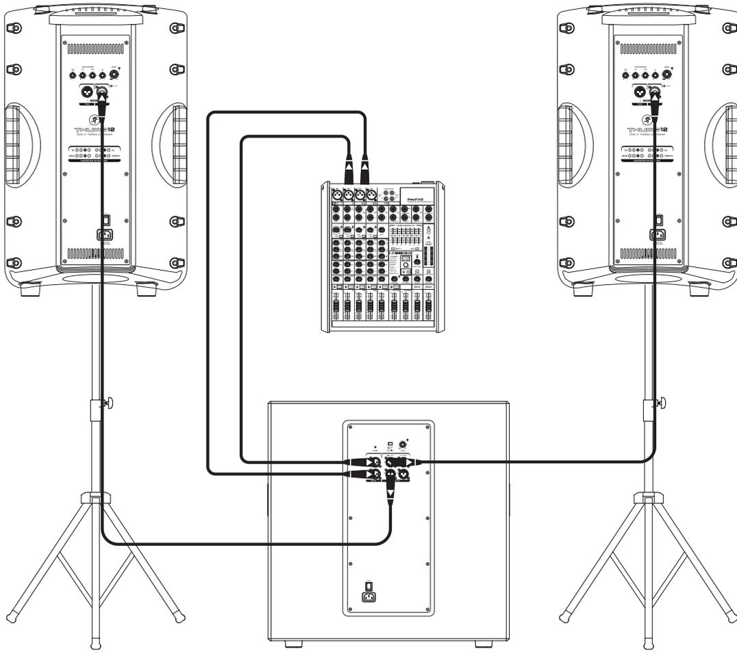
*In this example, a Thump18S subwoofer is connected to two Thump12 loudspeakers. It is a perfect setup for a small club.*
