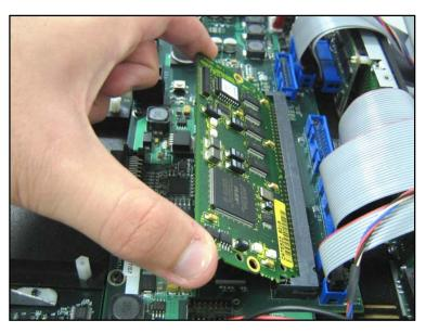
6. Slowly push the module down so that it is parallel to the main board. Two metal brackets on either side of the slot will snap into place over the edges of the module, holding it place. If the module does not move downwards, check the orientation of the board to make sure it is not upside down. **Do not force the module into place if it does not move easily.**
