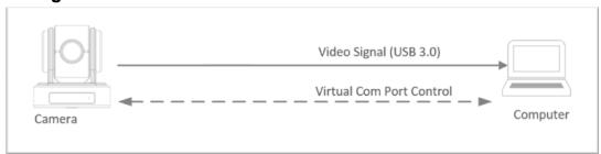
Before you use the virtual COM port, you need to install the driver onto your PC/Mac. You can download the driver (PL2303 Prolific Driver Installer v1.12.0) here: <a href="http://plugable.com/drivers/prolific">http://plugable.com/drivers/prolific</a> You can use this Virtual COM port to control the USB camera.
