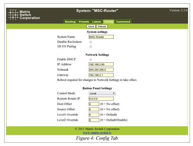
Figure 4 depicts the Config Tab as seen on a Router system beginning with Carina Series Firmware 5.3.0. Configuration fields vary depending on router features, firmware version and if the device is a Remote Panel.
