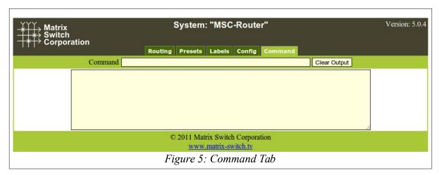
The Command Tab (Figure 5) provides access to the Mascot protocol interface. Commands are typed on the Command text entry line followed by pressing the Enter key to execute them. The results will be displayed in the text area below the command line. Clicking the **Clear Output** button will clear all command output in the lower area.
