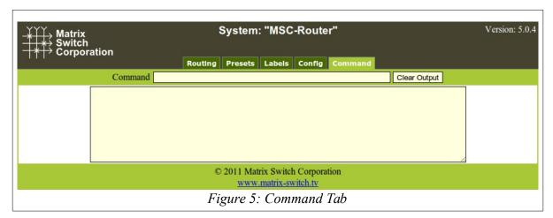
The Command Tab (Figure 5) provides access to the Mascot protocol interface. Commands are typed on the Command text entry line followed by pressing the Enter key to execute them. The results will be displayed in the text area below the command line. Clicking the **Clear Output** button will clear all command output in the lower area.
