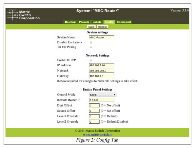
Figure 2 depicts the Config Tab as seen on a Router system beginning with Carina Series Firmware 5.3.0. Configuration fields vary depending on router features, firmware version and if the device is a Remote Panel.
