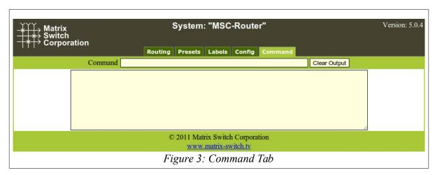
The Command Tab (Figure 3) provides access to the Mascot protocol interface. Commands are typed on the Command text entry line followed by pressing the Enter key to execute them. The results will be displayed in the text area below the command line. Clicking the **Clear Output** button will clear all command output in the lower area.
