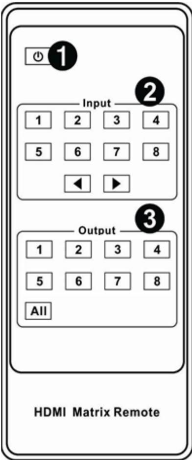
1. Power on /Standby: Press this button for powering on the matrix or setting it to standby mode.
