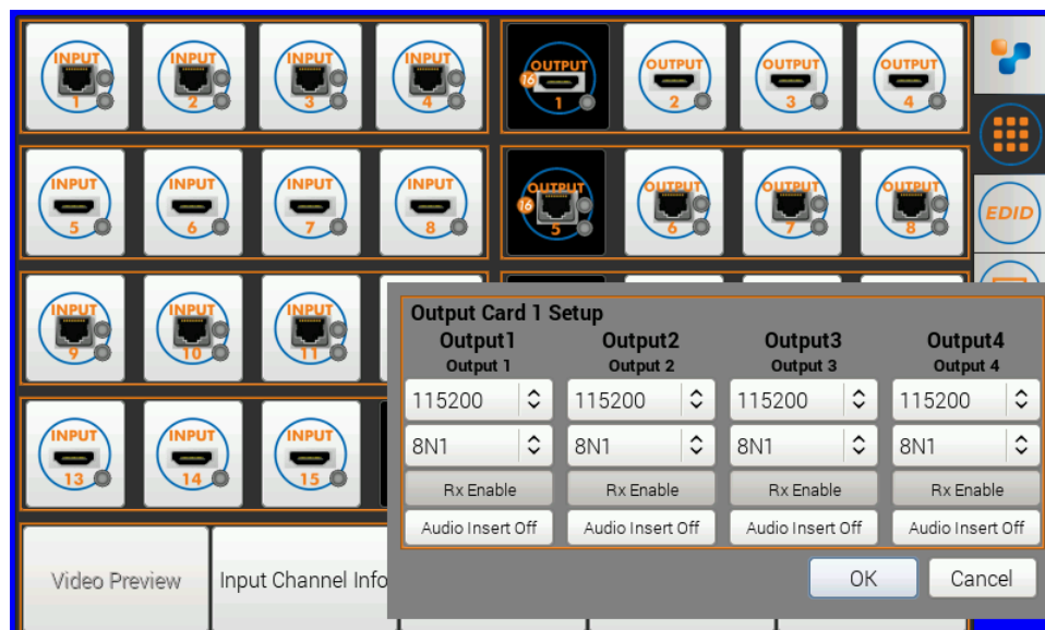
Figure 27: Output Card X Setup Dialog
