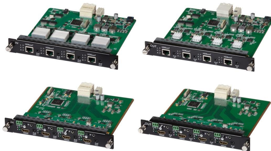
Figure 13: Input and Output Card Modules (Sold Separately)
