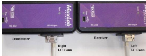
Figure 6 Connecting the Fiber Cable
