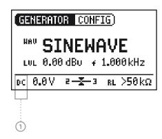
Unequal phantom voltages on Pin2 and Pin3 of the XLR cable indicate an error and will be displayed by the blinking of the phantom voltage display (DC).
