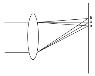
"Chromatic aberration" here refers to zoom factor chromatic aberration. Zoom factor chromatic aberration occurs since the diffraction ratio of a lens differs according to red (R)/green (G)/blue (B). Chromatic aberration on the lens itself is compensated for, but still remains in the periphery, in particular. Also, this chromatic aberration occurs on zoom lens due to a complex relationship between zoom ratio, iris and focal distance. In image terms, this is registration error.
