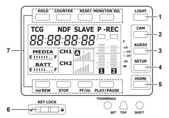
When the camera is turned on, the [HOME] screen is displayed. The status of the [HOME] screen at previous start-up is retained.
