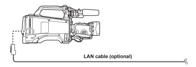
1 Connect the LAN cable to the <LAN> terminal on the rear side.
