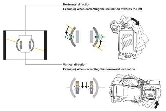
Orange lines will be displayed when inclined. Orange lines will be changed to green lines when there is almost no inclination. Inclinations will be displayed up to approximately ±45° in the horizontal direction, and up to ±30° in the vertical direction.
