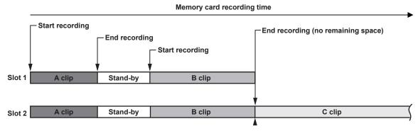
Selecting [ON] in the main menu → [RECORDING SETUP] → [SIMUL REC] will set the camera to simultaneous recording mode.
