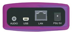
The Sx instrument Control panel provide the following connections.
