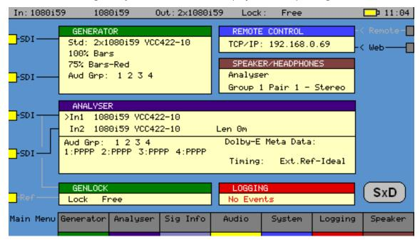
This page displays an overview for the system. It shows the video input and output standards and frame rate. The audio status for the generator shows which audio groups are being generated whilst the audio status for the input shows which groups are present and an overview of the channel status for each audio channel.
