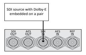
In this example, the SDI signal contains embedded audio with Dolby-E present on one or more audio pairs. The Sx instrument needs to lock its internal audio clock to the SDI signal (Generator – Genlock – Source = Input 1) and the Dolby Timing source should be set to SDI.
