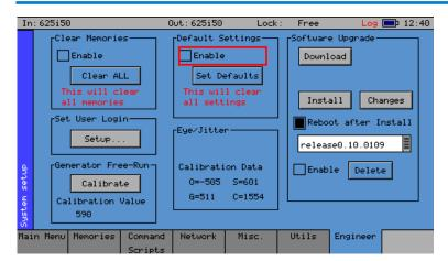
The Engineer menu is used to manage the Sx instrument and allows user access to be setup and the installation of new versions of software.
