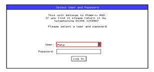
Using the User Login feature allows the Sx to be protected from un-authorised operation of the Front Panel controls. The prompt feature can allow a message to be displayed so that if the Sx instrument gets lost or stolen, someone finding it knows where to return it.
