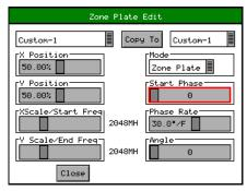
Mode - sets which type of Zone Plate is being produced. It may be Zone Plate (circular pattern) Grating (Linear horizontal or vertical grid) Sweep (Frequency sweeps from start to end Frequency)
