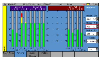
If AES inputs or outputs are present then these may also be metered. At the bottom of each meter is the current audio level for that channel in dBFs (decibels relative to 0dB full-scale).
