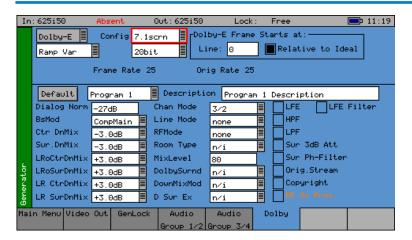
The Sx instrument Dolby software option allows generation of Dolby-E pre-encoded test signals to check that they are transferred transparently through the broadcast chain unaffected by routers/switchers, satellite links, etc.
