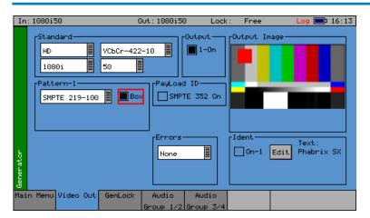
The Sx instrument can create video test signals for all supported SD and HD SDI output standards including the 3GHz standards at 1080p/50/59/60. It will support Y,Cr,Cb formats as well as RGB formats.
