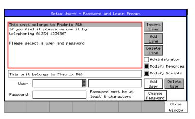
Once user log-in has been set up on your Sx a "Log out" button is added to the main menu which causes the log-in screen to be displayed. This may be used to protect a systems settings from being modified by other users. The system is still fully running while the log-in screen is visible.
