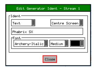
This dialogue allows selection of either a user defined bit map picture which has been downloaded into the 'Idents' directory of the Sx instrument or user defined text.
