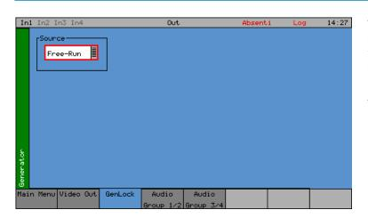
The SxE instrument can create video test signals that are either free-running or locked to a studio reference signal.
