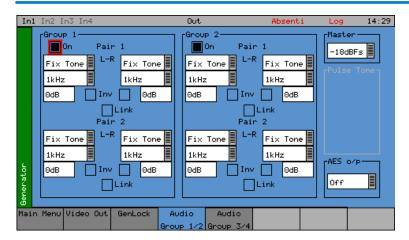
The Sx instrument can embed an audio signal on all 16 embedded audio outputs.
