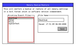
To export memories, select the Backup... button which will open a window to select the file to create. Existing files are shown and a new filename may be selected using the File Name edit box. Select the Save button to create the backup file. The filename created will have a .mem file extension.
