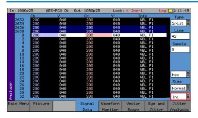
The Signal Data menu shows the video signal as a data stream in several formats as described below. In each mode, the data may be displayed in hexadecimal, decimal or binary formats. The binary format is not available in grid mode. The data may also be displayed as 10-bit or 8-bit format.
