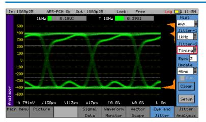
The Eye and Jitter menu displays the selected input in the form of an Eye Pattern Display.
