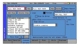
The Command Script option (PHSXOS) allows a series of pre-defined actions to be run through within the PHABRIX Sx using a script stored in internal memory.
