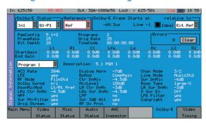
The Dolby E bit-stream Analyzer option (PHSXOBD-A) displays Dolby-E meta data present in a selected audio stream and determines whether the Dolby-E packet is timed correctly on the SDI video stream. The Dolby-E may be monitored from any of the SDI input embedded audio channel pairs or the AES input. Peak audio levels metering is also displayed.
