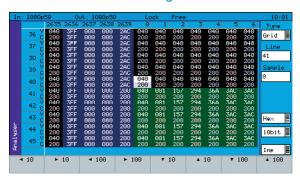
The SDI analysis option (PHSXOSD) provides the engineer with a detailed view of the data words contained within the SDI stream. This allows the analysis of complex faults and is particularly useful when determining compatibility issues between equipment and when debugging new product developments particularly in a R&D environment. Detail within the active SDI stream can be viewed with continuous update.
