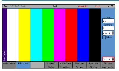
With Picture selected, the video picture is displayed in a window as a down-converted display. The picture will automatically view the horizontal or vertical blanking areas if the line or sample values are in the blanking area.
