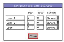
The Setup button and dialog allows user defined ANC packets to be configured.
