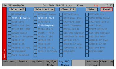
The Log ANC Status menu allows customisation of which ANC packets to log for changes in status (e.g. Present, Checksum Error, Missing, Parity Error). Individual check-boxes are provided to determine which packet DID/SDID combinations are logged.
