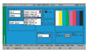
This option (PHSXOF) provides advanced formats include 4:2:2 YUV, 4:4:4 RGB and 4:4:4 YUV at 10/12 bit and 3G level A and B. For broadcast manufacturers this option allows rigorous testing of many more formats beyond the standard signals used in traditional broadcasting.
