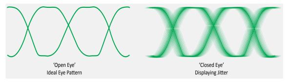
The Eye Pattern is formed by displaying the clock signal from the SDI data stream then superimposing a delayed version of the clock signal at exactly half way through the duty cycle (or unit interval) of the clock signal. This forms the recognisable eye shape.
