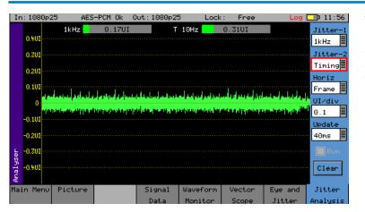
The jitter analysis display shows a trace of jitter amplitude versus time along with two jitter thermometers and has the following controls:
