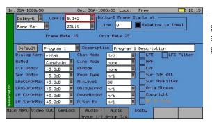
The PHABRIX Sx Dolby E bit-stream generator option (PHSXOBD-G) uniquely adds significant Dolby-E metadata generation features to the Sx range.
