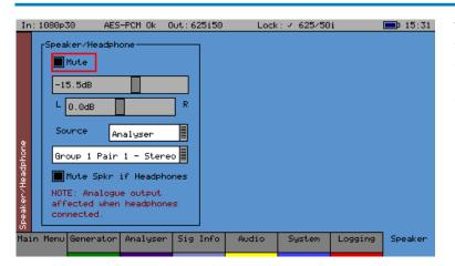
The Speaker menu controls which audio pair that can be heard on the loud speakers and headphone output of the unit.
