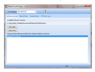
To connect to the instrument you will need to use the PHABRIX FTP client available from the PHABRIX website. This connects to the Sx unit using unit's IP address (as host name) with:
