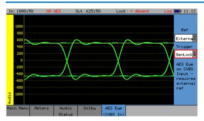
AES Eye menu allows an AES signal of  $75\Omega$  impeadance connected to the "PAL/NTSC (AES Eye) In" BNC connector to be displayed as an Eye pattern. This allows the amplitude and quality of the AES waveform to be seen and allows AES to reference locking to be checked
