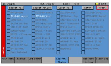
The Log ANC Status menu allows user-setup of which ANC packets to log for changes in status (e.g. Present, Checksum Error, Missing, Parity Error). Individual check-boxes are provided to determine which packet DID/SDID combinations are logged.
