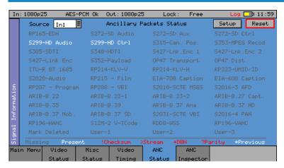
The ANC status menu shows which ANC packets are present on the SDI input and whether they have any errors. Each field is colour coded according to whether the ANC packet is present (White), missing (Grey), has errors (Red), or has previously had errors (yellow).
