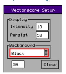
The Vectorscope Setup menu allows the intensity and persistence of the display to be adjusted. A colour wheel background can also be added.
