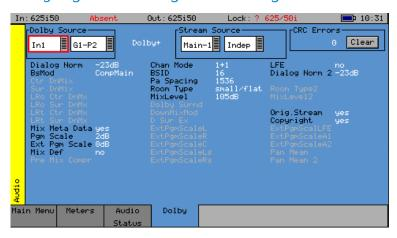
When Dolby Digital Plus metadata is analysed this displays the Main, Dependent and Independent program stream configuration and limited metadata that is sent with Dolby Digital Plus.
