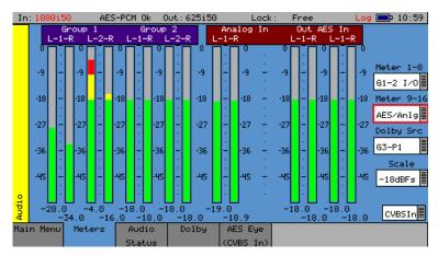
If AES or analogue inputs or outputs are present then these may also be metered. At the bottom of each meter is the current audio level for that channel in dBFs (decibels relative to OdB full-scale).
