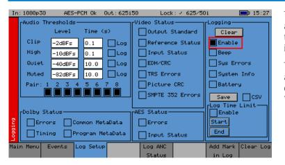
The Log Setup menu allows specific events to be tracked by the Sx instrument.
