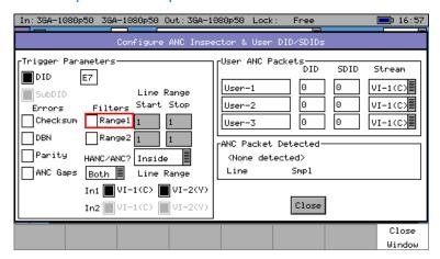
If the Setup button is pressed a dialogue box is shown to allow the ANC packet trigger parameters to be set. The trigger parameters allow only selected lines to be checked or excluded when checking for the presence of packets.
