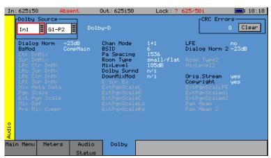
When Dolby Digital metadata is analysed this displays channel configuration and limited metadata that is sent with Dolby Digital.
