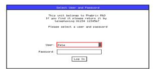
Using the User Login feature allows the Sx to be protected from un-authorised operation of the Front Panel controls. The prompt feature can allow a message to be displayed so that if the Sx instrument gets lost or stolen, someone finding it knows where to return it.
