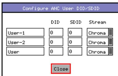
The Setup button and dialog allows user defined ANC packets to be configured.
