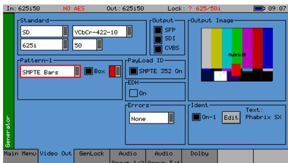
The Generator option (PHSXT-GEN) allows the creation of video test signals for analogue composite video, SD-SDI and HD-SDI video as standard. 3G-SDI, 2K SDI and Fibre video functionality can be purchased as additional options. The Generator option also allows the generation of both analogue and digital audio test tones and allows the unit to be locked to an external locking reference.
