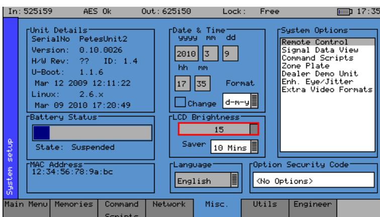
The Misc menu shows serial numbers, Sx instrument MAC address, version information and battery state. It also allows the date and time to be set and factory default settings to be recalled. The options security code is entered on this page if options are purchased.
