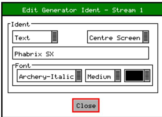
This dialogue allows selection of either a user defined bit map picture which has been downloaded into the 'Idents' directory of the Sx instrument or user defined text.
