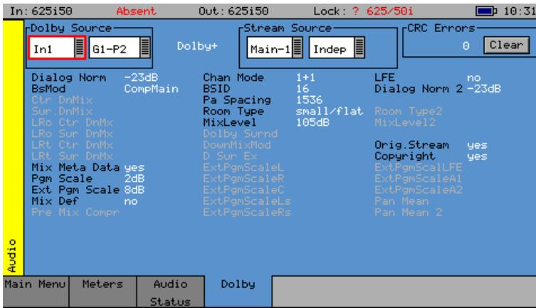
When Dolby Digital Plus metadata is analysed this displays the Main, Dependent and Independent program stream configuration and limited metadata that is sent with Dolby Digital Plus.
