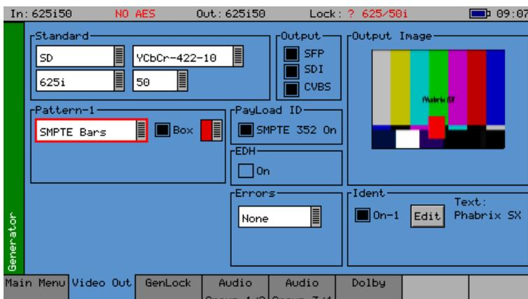
If the SxTAG instrument has the Generator option (PHSXT-GEN) installed it can create video test signals for all supported SD and HD SDI output standards including the 3GHz standards at 1080p/50/59/60. It will support Y,Cr,Cb formats as well as RGB formats.
