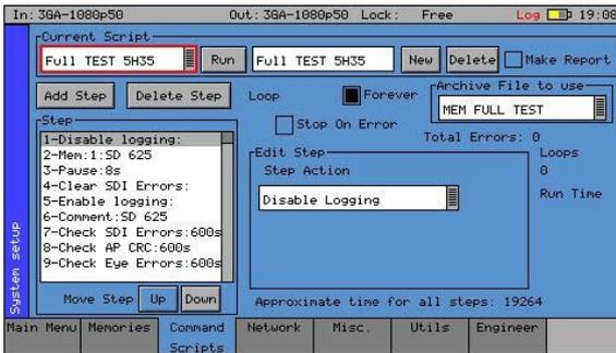
The Command Script option (PHXSOS) allows a series of predefined actions to be run through within the PHABRIX Sx using a script stored in internal memory.
