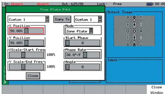
The Programmable zone plate option (PHSXOZ) adds a range of pre-programmed zone plate patterns along with user defined controls over several parameters which can be saved to custom buffers.
