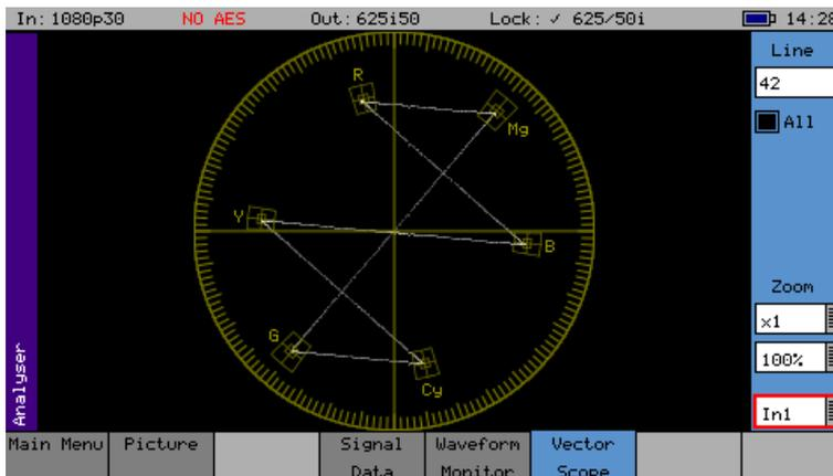
The Vectorscope menu displays the selected input in the form of a vectorscope. This may be set to show either the 100% bar positions or 75% positions. The colour bar position boxes will change according to the colour space for the current input video standard.
