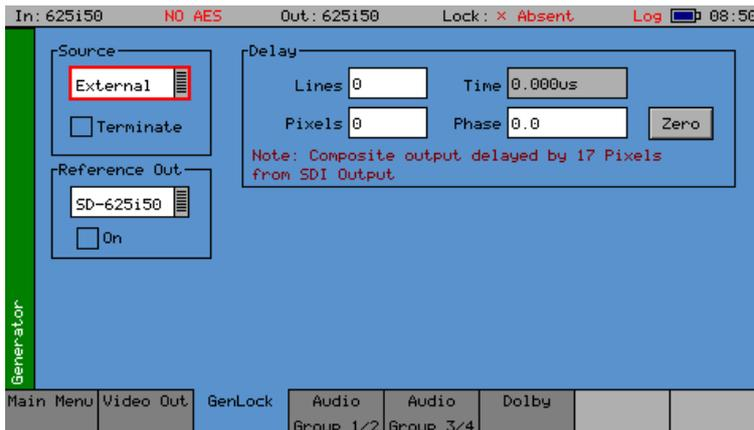
The unit can create video test signals that are either free-running or locked to a studio reference signal.
