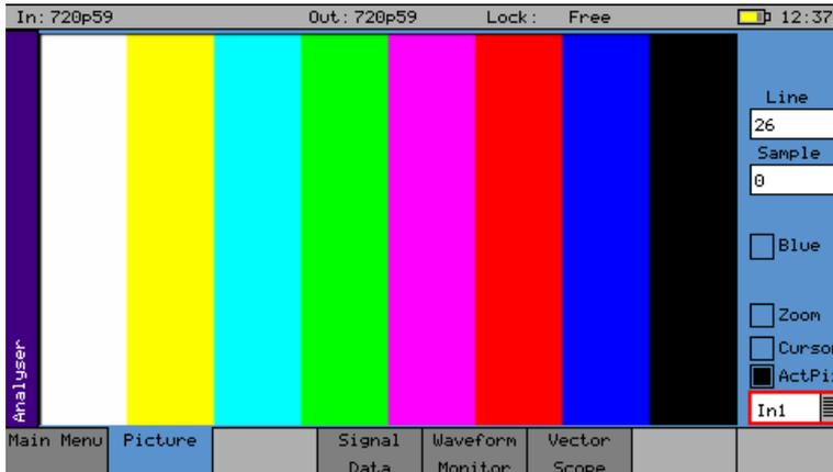
With Picture selected, the video picture is displayed in a window as a down-converted display.
