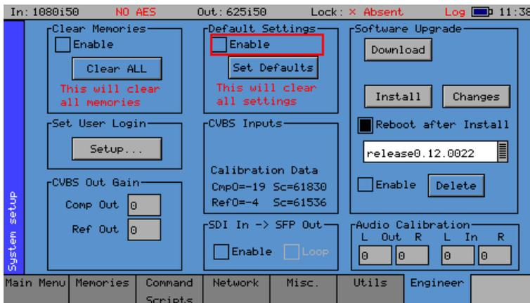
The Engineer menu is used to manage the SxTAG and allows user access to be setup and the installation of new versions of software.
