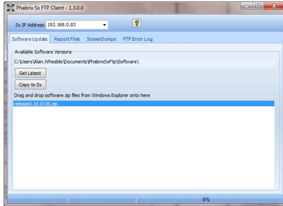
To connect to the instrument you will need to use the PHABRIX FTP client available from the PHABRIX website. This connects to the Sx unit using unit's IP address (as host name) with:
