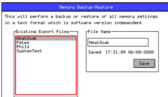
To export memories, select the Backup... button which will open a window to select the file to create. Existing files are shown and a new filename may be selected using the File Name edit box. Select the Save button to create the backup file. The filename created will have a .mem file extension.
