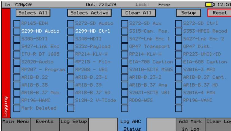
The Log ANC Status menu allows user-setup of which ANC packets to log for changes in status (e.g. Present, Checksum Error, Missing, Parity Error). Individual check-boxes are provided to determine which packet DID/SDID combinations are logged.
