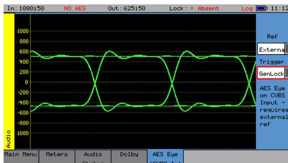
It can be difficult to check that the AES audio signal is correctly locked to the studio reference. The AES Eye Option allows the AES waveform to be displayed on the unit. If the studio locking reference is also connected to the unit, then the AES Eye waveform can be displayed locked to this reference.
