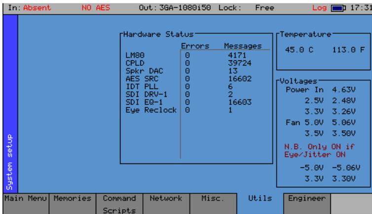
The Utils menu displays details of the Sx instrument's operating status and details the temperature and individual voltages. This menu also allows you to disable selected options.
