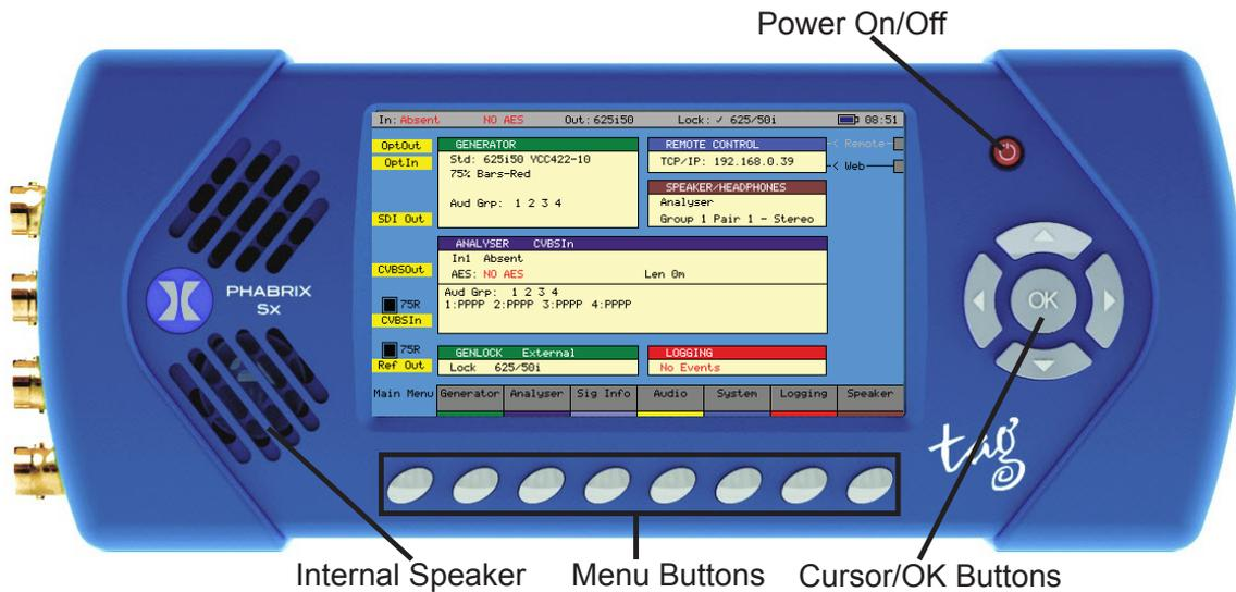
The front panel provides access to the TFT Display and menu system.
