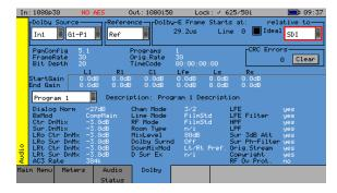
The Dolby bit-stream Analyzer option (PHSXOBD-A) displays Dolby E, Dolby Digital and Dolby Digital Plus metadata present in a selected audio stream and determines whether the Dolby E packet is timed correctly on the SDI video stream. The Dolby audio may be monitored from any of the SDI input embedded audio channel pairs or the AES input. Peak audio levels are also displayed for Dolby E.
