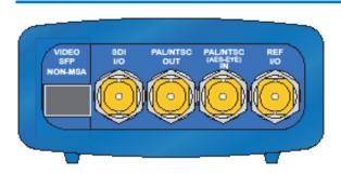
The SxTAG BNC panel provide the following connections.
