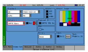
The Generator option (PHSXT-GEN) allows the creation of video test signals for analogue composite video, SD-SDI and HD-SDI video as standard. 3G-SDI, 2K SDI and Fibre video functionality can be purchased as additional options. The Generator option also allows the generation of both analogue and digital audio test tones and allows the unit to be locked to an external locking reference.
