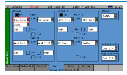
The Sx instrument can embed an audio signal on all 16 embedded audio outputs.
