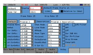
The PHABRIX Sx Dolby bit-stream generator option (PHSXOBD-G) uniquely adds significant Dolby E, Dolby Digital and Dolby Digital Plus metadata generation features to the Sx range.
