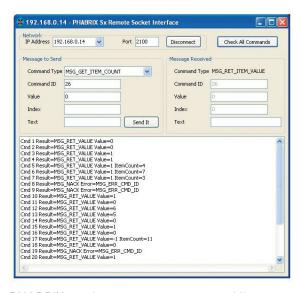
The Enhanced remote control option (PHSXOR) gives users full remote control of the unit via TCP/IP Sockets to allow any aspect of the unit to be modified or queried.
