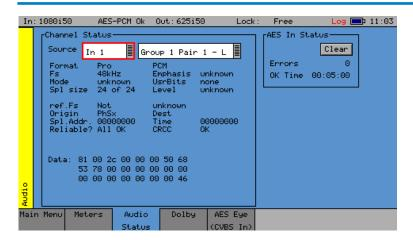
The Audio Status menu shows the Channel Status for the selected audio channel is displayed in decoded form as well as a hexadecimal dump of the bytes. The source may either come from the input signal or from the generator for comparison purposes.
