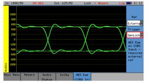
It can be difficult to check that the AES audio signal is correctly locked to the studio reference. The AES Eye Option allows the AES waveform to displayed on the unit. If the studio locking reference is also connected to the unit, then the AES Eye waveform can be displayed locked to this reference.
