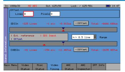
The Video Timing menu displays the relationship between the SDI and composite video inputs with respect to the locking reference input.
