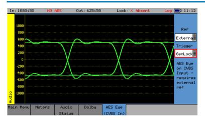
AES Eye menu allows an AES signal of  $75\Omega$  impeadance connected to the "PAL/NTSC (AES Eye) In" BNC connector to be displayed as an Eye pattern. This allows the amplitude and quality of the AES waveform to be seen and allows AES to reference locking to be checked
