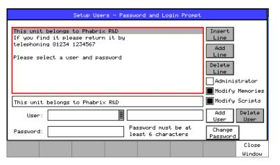
Once user log-in has been set up on your Sx a "Log out" button is added to the main menu which causes the log-in screen to be displayed. This may be used to protect a systems settings from being modified by other users. The system is still fully running while the log-in screen is visible.
