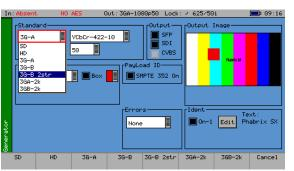
This option (PHSXO-2K) supports the new SDI practice for HD and 3G Level A and Level B signal transfer of 2K advanced formats including 4:2:2 Y'C'bC'r, 4:4:4 R'G'B' and 4:4:4 Y'C'bC'r at 10/12 bit as well as 4:4:4 X'Y'Z' at 12-bit. For broadcast manufacturers this option allows rigorous testing of many more formats beyond the standard signals used in traditional broadcasting.
