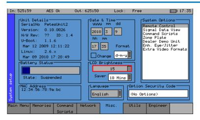
The Misc menu shows serial numbers, Sx instrument MAC address, version information and battery state. It also allows the date and time to be set and factory default settings to be recalled. The options security code is entered on this page if options are purchased.
