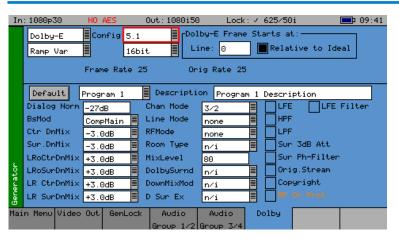
The Sx instrument Dolby Generator software option allows generation of Dolby-E, Dolby Digital and Dolby Digital Plus pre-encoded test signals to check that they are transferred transparently through the broadcast chain unaffected by routers/switchers, satellite links, etc.
