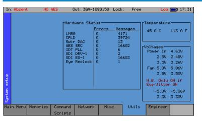
The Utils menu displays details of the Sx instrument's operating status and details the temperature and individual voltages. This menu also allows you to disable selected options.
