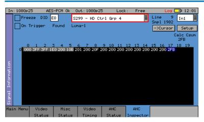
The SDI Data Option allows Ancillary data packets to be detected and checked for errors.
