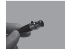
TA4-F for most Shure® wireless transmitters.
