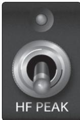
**High Band Peak:** When the Peak switch is engaged, the high band of the EQ becomes a standard peak filter with a fixed Q of 0.6. When it is disengaged, the high band is a shelving filter.
