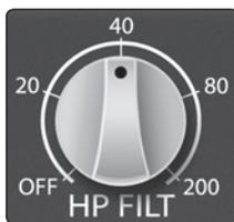
**High Pass Filter:** The high-pass filter's frequency threshold can be set at 20 Hz, 40 Hz, 80 Hz, or 200 Hz, or it can be turned off completely. The slope of the filter is -12 dB/octave.
