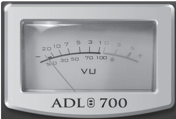
**VU Meter:** The analog VU meter displays the ADL 700's output level. When the Meter – GR switch is enabled, the VU meter will show the amount of gain reduction being applied by the compressor.
