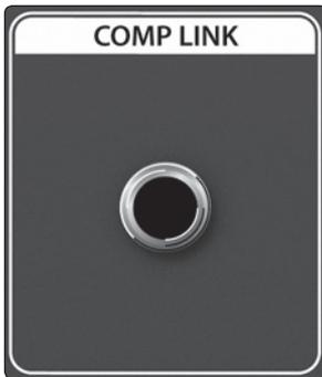
**Comp Link:** Use this TRS connection to link the compressor stage of two ADL 700s.
