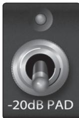
**-20 dB Pad:** The pad provides 20 dB of attenuation for the microphone preamp only.
