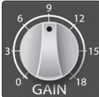
**Make-up Gain:** Compression usually results in an overall reduction of level. The Make-up Gain knob allows you to restore the pre-compression level. You can adjust Make-up Gain from -0 dB to +18 dB.
