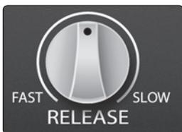
**Release:** Sets the release of the compressor, which is the time the compressor takes to return the gain reduction back to zero (no gain reduction) after the signal level crosses below the compression threshold. The compressor release time ranges from 40 ms (Fast) to 500 ms (Slow).
