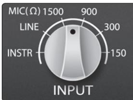
**Input Source Select.** The Input Source Select switch allows you to choose among all signal sources that you have connected to the ADL 700 inputs. It patches the selected input through the signal chain, completely bypassing the other two inputs. The Input Source Select switch also provides a choice of four mic-input impedances: 1500Ω, 900Ω, 300Ω, and 150Ω.
