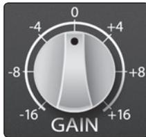
**Low Band Gain:** Sets the attenuation or boost of the EQ's low band. The gain can be set between -16 and +16 dB.
