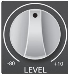
**Level:** Adjusts the overall output volume of the ADL 700 from -80 dB to +6 dB
