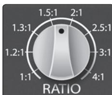
**Ratio:** The Ratio control sets the compression slope, which is the relationship between the output level and the input level. For example, if you have the ratio set to 2:1, then for every 2 dB of level increase above the threshold, the compressor's output will only increase 1 dB. The ratio can be set from 1:1 to 4:1.
