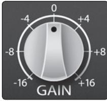
**High Mid Band Gain:** Sets the attenuation or boost of the EQ's high-mid band. The gain can be set between -16 and +16 dB.
