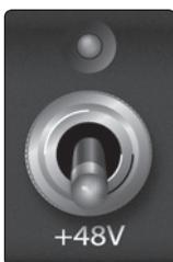
**+48V.** The 48-volt phantom power, supplied by way of the XLR input, provides power for condenser microphones and other devices requiring continuous power. This power is supplied at a constant level to prevent any signal degradation.
