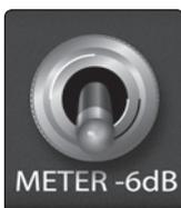
**Meter -6 dB:** This switch offsets the VU meter by 6 dB, which can help you meter loud input sources if your VU meter is "slamming" or pegged.
