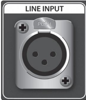
**Line Input:** This balanced XLR connection can be used for line-level devices such as keyboards, drum machines, and sound modules. You can also use the line inputs on two stereo-linked ADL 700s to give a stereo mix an extremely full, rich character. To use this input, turn the Source Select switch to the Line position.
