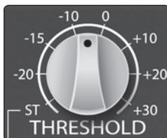
**Threshold:** Sets the threshold of the compressor. When the signal's amplitude (level) exceeds the threshold setting, the compressor engages. Turning the knob counterclockwise lowers the threshold so that compression begins at a lower amplitude, and more of the input signal becomes compressed (assuming you have a ratio setting greater than 1:1). The threshold can be set from -20 to +30 dBu.
