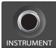
**Instrument Input:** The ¼" TS connector on the front panel is for use with a passive instrument (guitar, bass, etc.). To use this input, turn the Source Select switch to the "Inst" position.
