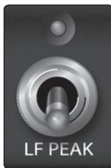
**Low Band Peak:** When the Peak switch is engaged, the low band of the EQ becomes a standard peak filter with a fixed Q of 0.6. When it is disengaged, the low band is a shelving filter.
