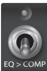
**EQ>Compressor:** When the EQ>Compressor switch is engaged, it places the EQ before the compressor in the signal path. When it is disengaged, the signal passes through the compressor before passing through the EQ.
