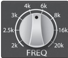
**High Band Frequency:** Sets the center frequency of the EQ's high-frequency band. You can adjust the center frequency from 2 kHz to 20 kHz.
