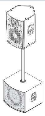
All full-range StudioLive loudspeakers are equipped with 35 mm pole socket that allows the speaker to be mounted on a speaker stand or on a pole over an 18sAl subwoofer. This pole socket allows for straight 90° vertical mounting or for tilting the full-range loudspeaker down 10° while on a pole.
