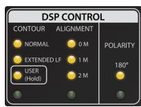
**DSP Contours.** Your 18sAl Subwoofer is equipped with two DSP contours. These contours change the character of your StudioLive loudspeaker in a fundamental way, adjusting FIR filters, alignment, and crossover settings to customize your loudspeaker for one of two applications:
