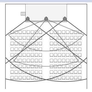
An LCR system is a stereo system with a center speaker added. This configuration allows panning and adds depth to the acoustic image. This type of system will provide more control than a basic stereo system and is ideal in situations where music and speech intelligibility are equally important.
