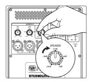
11. If more output level is required, turn the Speaker level knob clockwise. This is the master level control for your loudspeaker. It controls the mixed signal of the Mic and Line inputs.
