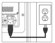
1. With the power switch in the Off position, connect the locking IEC plug to the IEC socket connection on the back of the loudspeaker and plug it into a grounded AC outlet or surge protector.
