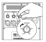
9. Turn the Speaker level knob on your full-range loudspeakers to the 12 o'clock position.
