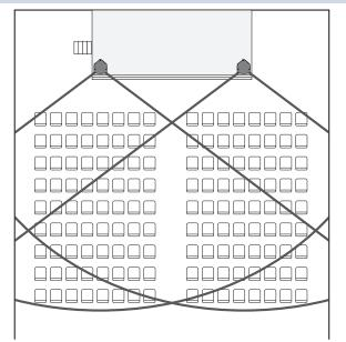
A stereo system allows panning and adds depth to the acoustic image. This is good for speech reinforcement and greatly enhances live or prerecorded music. Locate speakers to give the best horizontal coverage. Ensure that the listeners are well covered by the pattern.
