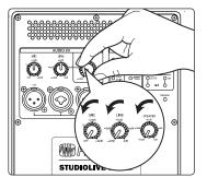
2. Turn the Mic, Line, and Speaker level knobs fully counterclockwise, to the lowest position.
