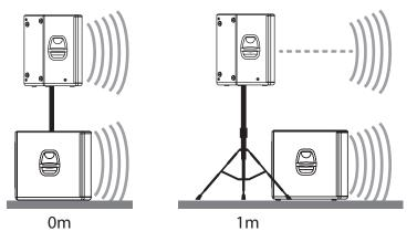
**OM.** Select this setting when the full-range system is directly over the subwoofer (i.e., mounted atop using the SP1BK sub-pole accessory). No delay is added to the subwoofer amplifier output.
