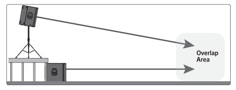
Find the spot in the room where coverage from the main speakers and the subwoofers overlap. Measure the distance from the overlap area to each speaker location. Subtract the smaller distance from the larger. Divide that number by 1,100 and apply that delay value to the speaker that is closest. Keep in mind that the overlap area may be behind FOH.
