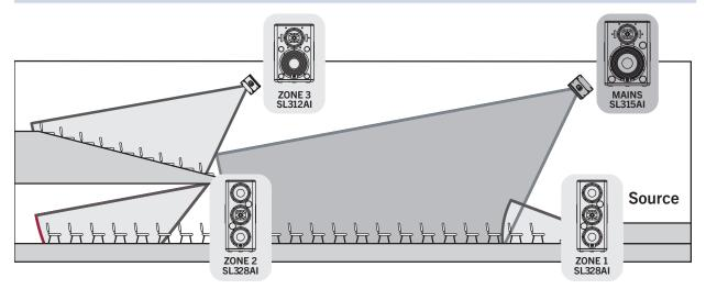
The goal in a complicated system with loudspeakers distributed throughout the venue is to delay each satellite system to its counterpart in the main system (e.g., the left front fill to the left FOH loudspeaker).
