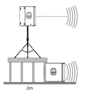
**2M.** Select this setting when the subwoofer is about two meters from the full-range loudspeaker—typical when the full-range system is on the stage and the subwoofer is on the floor. A delay of about 5.9 ms is introduced to the signal that is output through the subwoofer amplifier.
