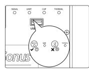
10. Both the Microphone and Line inputs should be set so that the green Signal LED is illuminated most of the time, but the red Clip LED illuminates only with the highest transient peaks or not at all.
