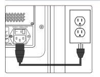
1. With the power switch in the Off position, connect the locking IEC plug to the IEC socket connection on the back of each loudspeaker and plug it into a grounded AC outlet or surge protector.
