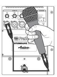
3. If you're using the StudioLive full-range loudspeaker as a mixer, connect a microphone to the Mic input with a standard XLR cable.
