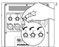
Turn the Mic, Line, and Speaker level knobs on your full-range loudspeakers fully counterclockwise to the lowest position.
