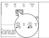
12. The line-level inputs should be set so that the green Signal LED is illuminated most of the time, but the red Clip LED illuminates only with the highest transient peaks or not at all. If your line-level source is clipping the inputs on your 18sAl, you will need to turn down the source's output level.
