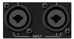
**Line Inputs.** The 18sAI features two line-level inputs. These balanced combo connections are provided to connect your subwoofer to a StudioLive digital mixer or other mixing console. The line inputs will accept up to a +24 dBu source before clipping.
