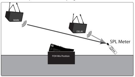
Once you have positioned and delayed your satellite system, use an SPL meter to match the output of the main and delay systems at the measurement point. If you are standing 20 feet from the left side of the main system and 30 feet from the left side of the delay system, and if the output of the main system is 85 dB, the output of the delay system should also be 85 dB.
