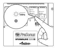
13. If more high-frequency output level is required, turn the Speaker level knob clockwise on your full-range loudspeakers. In most cases, the level should be set the same on both loudspeakers.
