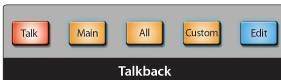
The CS18AI will automatically assign Input 1/TB as the talkback source for the connected RM mixer. This can be routed to the aux outputs and to the mains.
