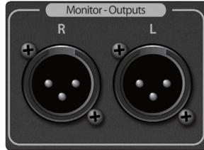
The monitor outputs are balanced XLR-M jacks and are convenient for control room monitoring when the CS18AI is used to control Studio One or for monitoring in broadcast applications. The signal routed to these outputs is the same as that appearing at the headphone outputs.
