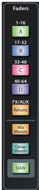
The CS18AI has eight layers for accessing all available channels for control. Using the buttons in the Faders area you can switch between the channel layers. Once a layer has been selected, it remains active on the channel strips until you navigate to another layer.
