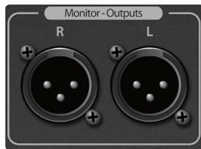
9. **Monitor Outputs.** Electrically balanced XLR-M jacks provide the monitor outputs for the control surface. The level is controlled with the top-panel Monitor knob. The source mirrors the headphone outputs.
