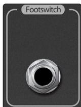
6. **Footswitch Input.** A 1/4-inch jack supports a momentary footswitch. The target for footswitch control is set in the Master Control touchscreen.
