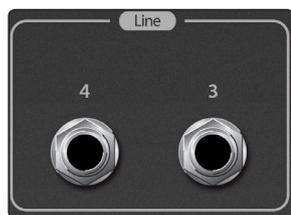
The CS18AI rear panel includes two TRS Line Input jacks. These jacks provide additional line inputs for sources from front-of-house, such as 2-track or computer playback. On a StudioLive RM-series mixer connected to the CS18AI via AVB, these two inputs show up as digital returns 33 and 34, which appear on the Returns layer as Dig Ret.
