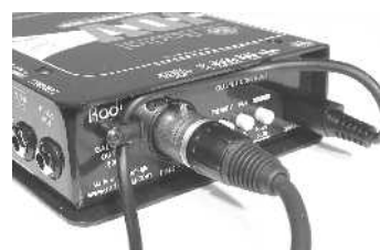
The JDV's strain relief in action.
