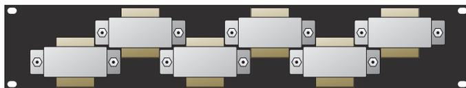
MT6 rear panel with six transformers installed.
