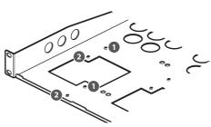
2 is for use with the unit installed flush against the front panel.
