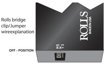
Rolls utilizes a way of switching with a three pin jumper wire system attached to the P.C.B. It uses an external bridge clip to act as a switch for changing between two preset unit options.
