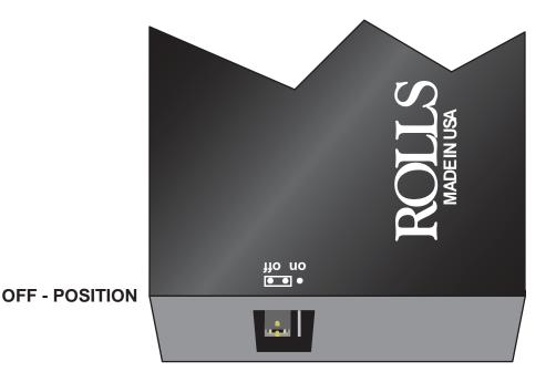
Rolls utilizes a way of switching with a three pin jumper wire system attached to the P.C.B. It uses an external bridge clip to act as a switch for changing between two preset unit options.
