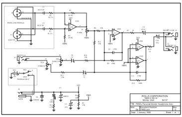
SPECIFICATIONS Max Input Level: -20 dB XLR, 40 dB monitor Output Impedance: 10 Ohms Gain: 15 dB 1/4", 50 dB XLR Bandwidth: 20 - 20 kHz S/N Ratio: 90 dB Power: 9 - 18 VAC/DC Size: 3" x 2.5" x 1.25" (7.6 x 6 x 3.2 cm) Weight: 1 lb (.45 Kg)
