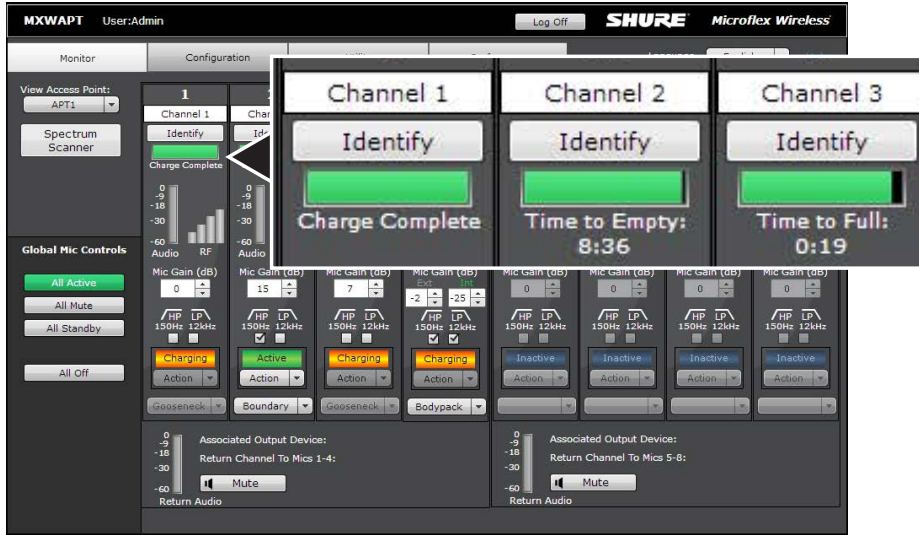
Monitoring Battery Charge Status
