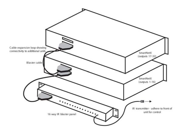
IR Blaster unit connected to SmartNet-V unit
