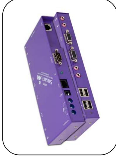
Use CAT5 cable to broadcast high resolution SXGA, Stereo Audio, RS232/IR and USB 1.1 up to 275ft.
