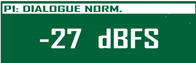
Fig 1-9: RB-DEED8 Metadata Status Screen showing the Dialogue Normalization parameter.
