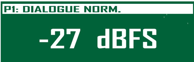
Fig 1-13: RB-DEED8 Metadata Status Screen showing the Dialogue Normalization parameter.
