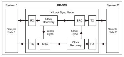
Fig 4-2: RB-SC2 X-Lock Sync Mode
