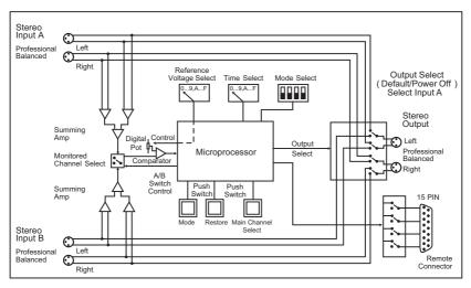
Fig 9-2: RB-SD1 System Block Diagram
