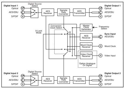
Fig 4-4: RB-SC2 System Block Diagram
