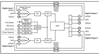
Fig 10-2: RB-DSD1 System Block Diagram
