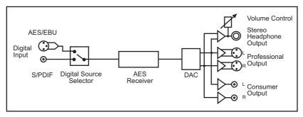
Fig 5-2: RB-DAC1 System Block Diagram
