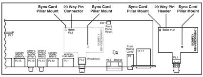
Fig 4-3: RB-SC2 Optional Video Sync Installation
