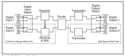
Fig 6-2: RB-SP1 System Block Diagram
