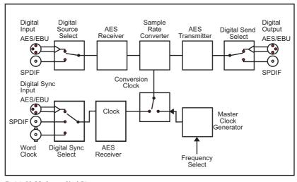
Fig 3-2: RB-SC1 System Block Diagram
