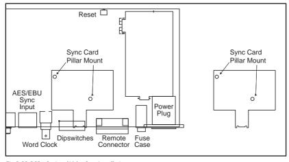
Fig G: RB-DSD1 Optional Video Sync Installation
