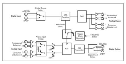
Fig 1-2: RB-ADDA System Block Diagram
