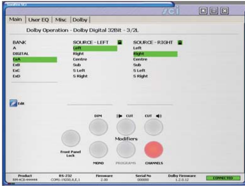
Fig 6-5: Sci Main Screen Showing Dolby Digital Monitoring
