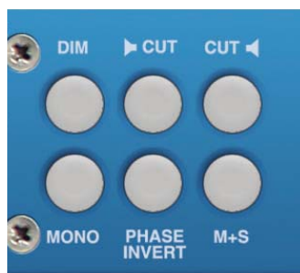
Fig 1-15: RM-2S4 & RM-2S10 Modifier Switches
