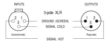
Mono input channel's mic input, Stereo input channel's mic inputs, Master section: T/B mic. Master section: Mix L, Mix R, Mix Mono, Grp 1-4 Aux 1-4, Matrix 1-2.
