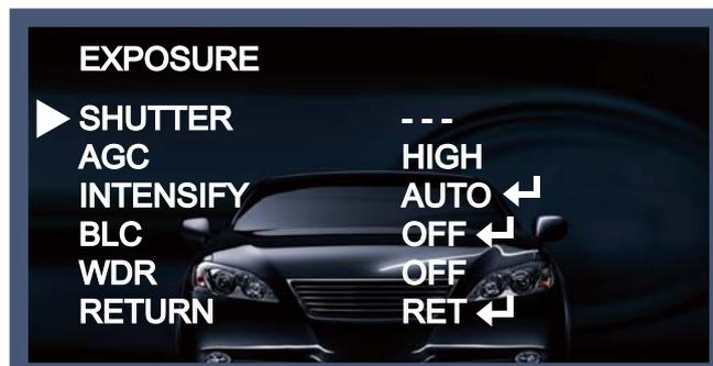
◆ Electronic Shutter : DC lens is launched with the setting of 1/60 and the manual lens is launched with the setting of Auto shutter, but the shutter speed can be adjusted from 1/60 to 1/100,000.
