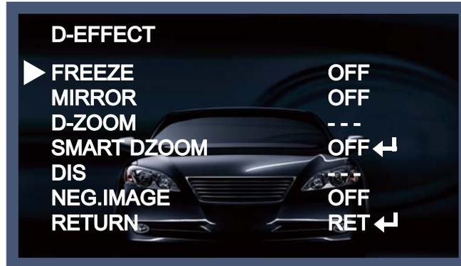
→ FREEZE : The image of the monitor is paused temporarily by this function.
