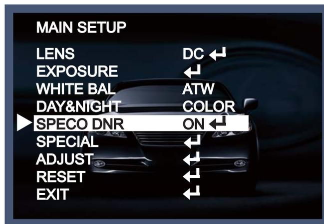
3. Adjust the most available proportion of compensation with the ambient environment by changing the SPECO DNR mode into On and pressing the Set button.
