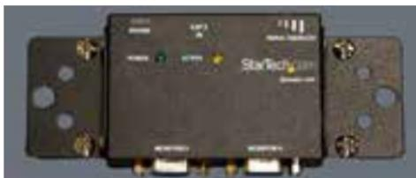
6. Using the Monitor Out ports, connect the Receiver to the display. Note that each Receiver unit can be connected to two separate displays simultaneously. To connect two monitors, simply connect a VGA cable from the second Monitor Out to a second display.
