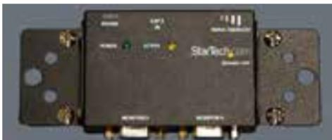
5. Using a standard UTP cable with RJ45 terminators on each end, connect the Cat5 OUT port provided by the Transmitter Unit to the Cat5 IN port provided by the Extender Unit.
