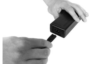
3. **OPTIONAL:** Connect the small, cylindrical power connector (splits off from LP4 connector) provided by the Switching Power Adapter to the corresponding power port on the Hard Drive Adapter. This is only required if the Hard Drive Adapter cannot draw enough power directly from the USB port.
