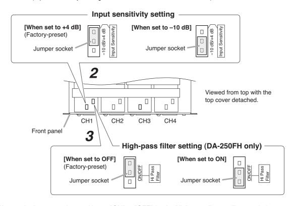
Step 4. Change the jumper socket position to "ON" or "OFF" for the High-pass filter as illustrated above. (DA-250FH only)
