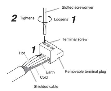
**Tip**Recommended slotted screwdriver type: Screwdriver with blade that is 3 mm (0.12") in width
