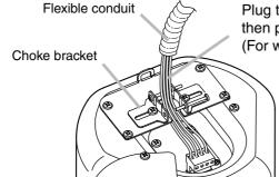
Plug the wired input connector into the speaker's socket, then pull the speaker cable from the choke bracket. (For wiring the input connector, refer to p. 12.)
