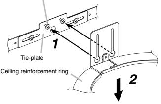
Fit closely to the back surface of the ceiling panel.
