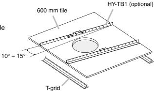
**Step 3.** Place the supplied reinforcement ring on the ceiling panel.
